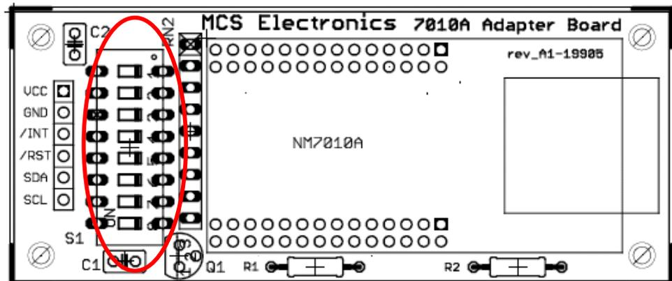
The TWI/I2C slave must have a unique address. The LS bit is used to indicate Read or Write and cannot be set. Therefore, it is not connected to the DIP switch. As DIP switches with seven switches are hard to find, the PCB is designed so that you can use a DIP switch with 7 or 8 switches. The switch number indicated with “8” is not connected. When you choose to insert a DIP with 7 switches, make sure that position 1 matches position 1 on the PCB and that position 8 on the PCB remains open/unused.
