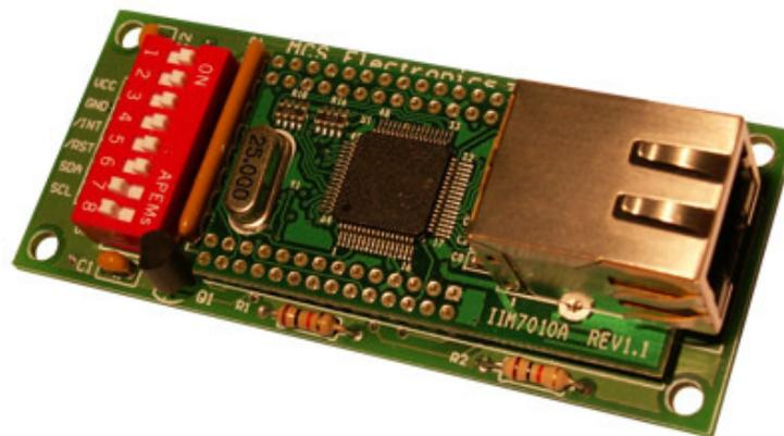
The shown address is A7=1, i.e., &B10000000 = &H80 = 128(dec). The switch at position 8 may be in any position since it is not connected.
